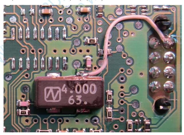
Then solder red wire of our cable for power supplying.
