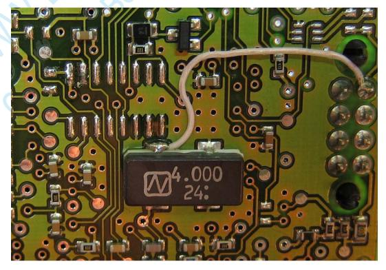
Find resistor on **RESET** line and make a jump on it for good communication. (you can keep this jump even after reading/writing finishing).
