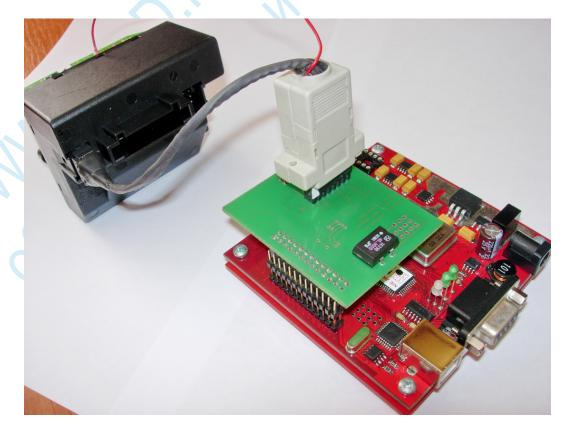
Start the programmer software and press DEVICE button.
