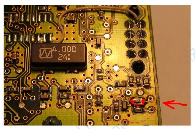
Then solder red wire of our cable for power supplying.
